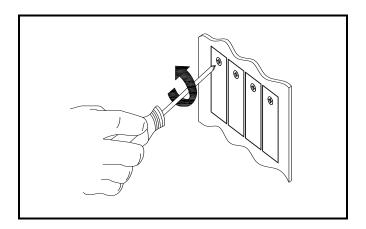
Step 2: Insert KCU-40 module into the slot.
