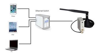
When KCU-40 is connected with the Internet, it'll automatically link to KUTAI communications server and waiting to connect to remote control devices.
